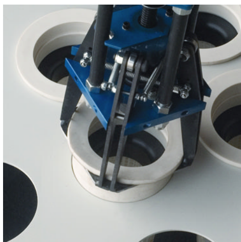
This sequence shows how the Grapoid effortlessly breaks the especially tight seal of a pleated bag, allowing easy removal.
