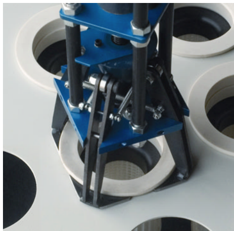
The Grapoid™ is operated by a standard cordless drill, pneumatic wrench, or hand tool. It can be equipped to remove both pleated and felt bags.
