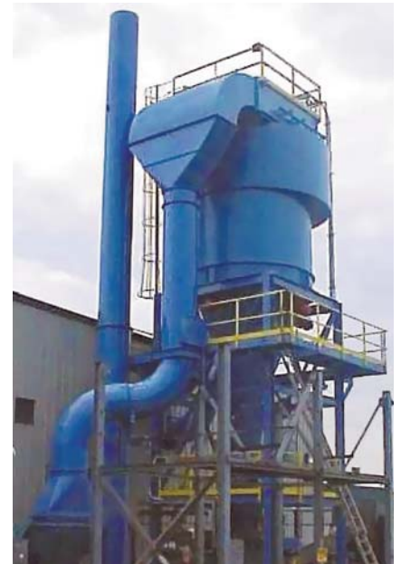
Tangential inlet design for low bulk density dust
