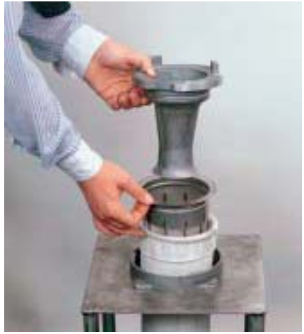
Bag Fastening in Tube Sheet
